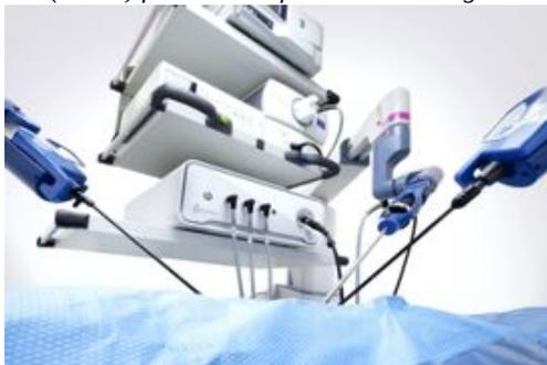
*Image Caption: The Senhance Surgical System pictured with the latest ISU model that includes expanded augmented intelligence features such as 3D measurement and enhanced camera control.*
