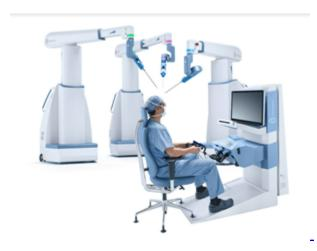
Senhance Surgical System is the first of its kind digital laparoscopic platform providing surgical assurance through haptic feedback, eye-tracking camera control, 3D visualization and 3mm instruments.
